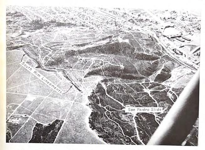
Figure 2. Oblique aerial photograph of southwestern Otay Mesa showing South Rim lineaments and the San Ysidro slide (view to south with Tijuana, Mexico in upper portion of photo).
