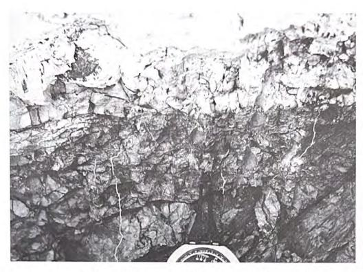
Figure 5. Exposure of sheared claystone bed in upper portion of the Beyer School cut slope. Light colored material near top of photograph is a well-cemented calcareous siltstone. The shear zone is approximately three inches thick and lies just above the Brunton compass.
