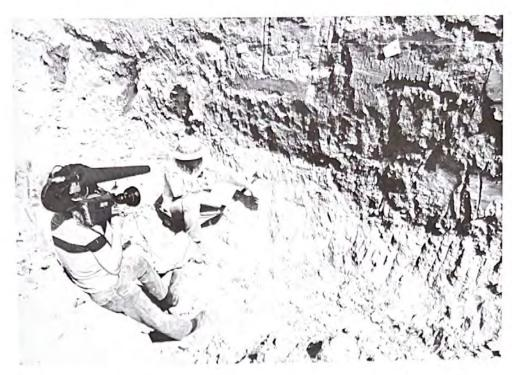
Figure 7. R. Dowlen pointing out the main trace (trace no. 1 on Figure 6) of the La Nacion fault. Dark colored Holocene paleosol lies unbroken over the lighter-colored bedrock.
