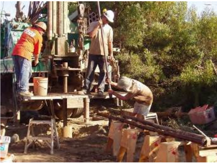
Figure 3B. Core samples are taken from selected depths using a wire-line device. Cores help correlate geologic layers.
