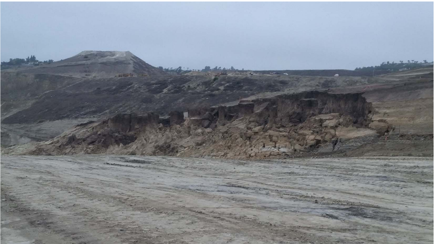
Backcut failure along a bedding plane shear in the Puente Formation.
