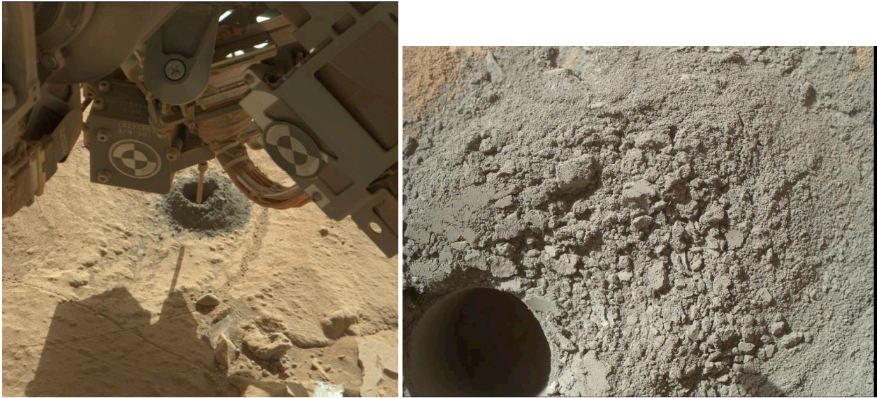
Windjana Drill target – MCAM taking a picture of MAHLI taking a picture of the drill hole and tailings on left; MAHLI image of drill hole and tailings on right.
